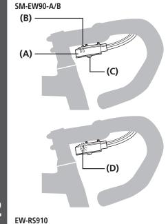
Press the button at junction A until the button LED illuminates in order to switch from gear shifting mode to adjustment
