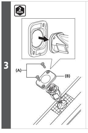
Insert junction A into the frame and attach the holder plate.
