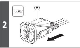
Connect the electric wires to junction A.
