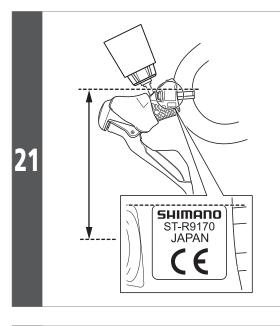
Make adjustments, such as changing the angle of the handlebar, so that the side of the bracket indicated in the illustration is parallel to the ground.
