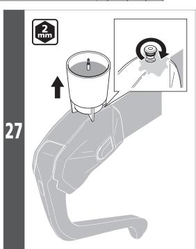
Remove the oil funnel while still plugged with the oil stopper.
