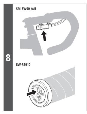
Press the button at junction A until the red LED turns off in order to switch from rear derailleur adjustment mode to gear shifting mode.
