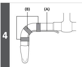
Temporarily secure the outer casing to the handlebar (by using tape or a similar material).
