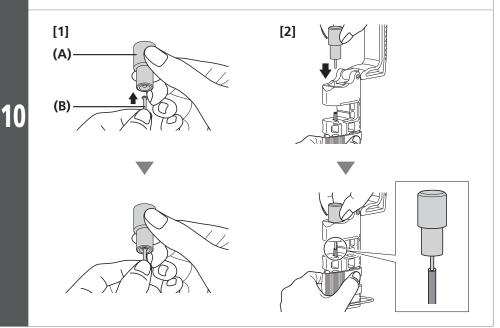
Grip the lever on the tool to insert the connector insert into the brake hose, as shown in the
