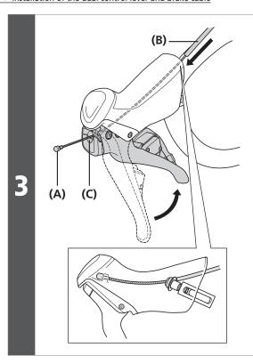
Depress the lever as if to brake and pass the brake cable through.
