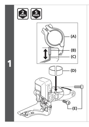
Install the clamp band to the front derailleur.
