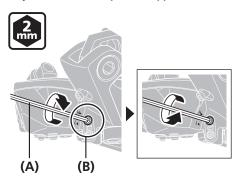
Shift to the smallest sprocket, and then tighten the top-side stopper bolt until it touches the left link at the position where the rear derailleur stops.
